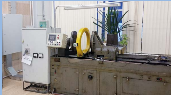
Example of modernization of magnetic flaw detector УМДЭ-10 000
