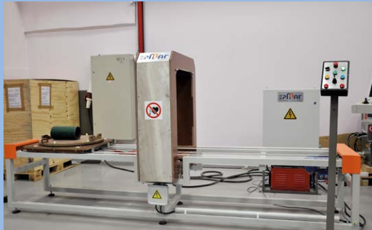
Semi-automatic device for demagnetization of parts in the conditions of manufacturing, repair and maintenance
