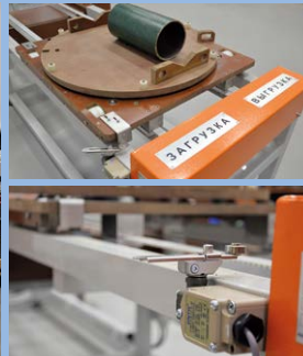
Semi-automatic device for demagnetization of parts in the conditions of manufacturing, repair and maintenance
