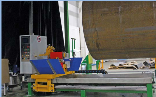
System of magnetic particle inspection of pipe ends
