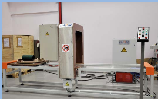
Semi-automatic device for demagnetization of parts in the conditions of manufacturing, repair and maintenance
