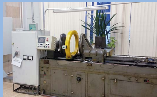
Example of modernization of magnetic flaw detector УМДЭ-10 000
